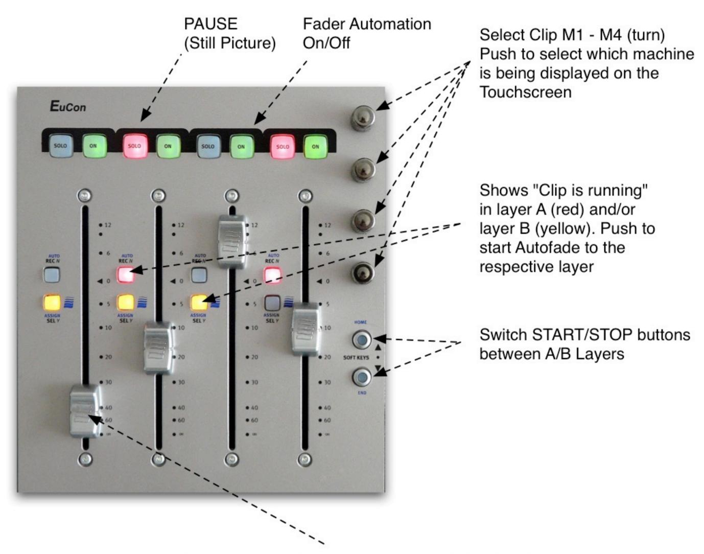
Four touch sensitive faders, interrupt Autofade when touched. Operation of jog-wheel and buttons around it correspond to the last touched fader (or started/stopped machine, see next pages).
