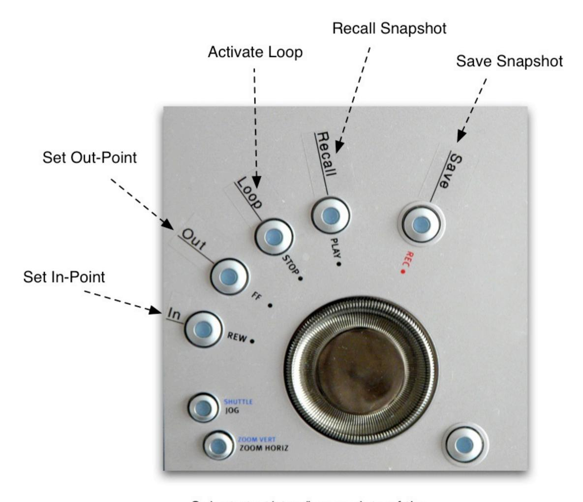
Select start/stop/loop points of the last selected Machine (layer A) via Jog-Wheel
